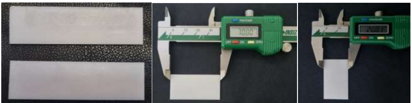
Figure 4: Zirconia samples fabricated for surface Gloss evaluation
