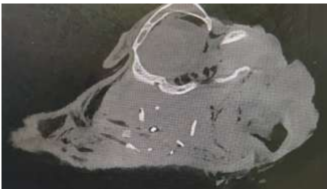
Figure 5: CBCT view of sheep's head. Bone particles and metal objects are easily detectable. Some metal artifact is present.
